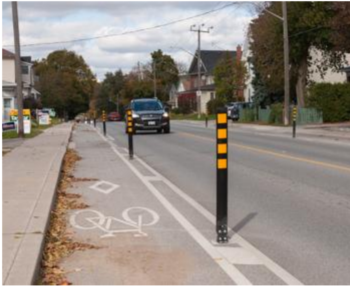
PHYSICALLY SEPARATED BIKE LANE IN ONTARIO
